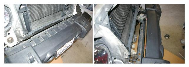
*Note: The black plastic piece can be a little tough, but once you have removed the fasteners you can twist the plastic piece and pull it out to the side.*
